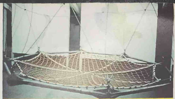
1:7 Model of Giant Algae System Clean Air Rig, prepared for Laminaria (as opposed to the much-larger Macrocyctis), suitable for the areas indicated behind: East China Sea/Yellow Sea Basin; Kuroshio Current. Ocean Earth Development Corporation
